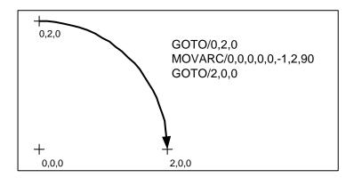
In this example, the start point of the arc is 0,2,0. The arc center is at 0,0,0 and the cylinder axis is 0,0,-1 ( the -1 signifying that the cutting direction is clockwise; a positive vector signifies counter-clockwise direction, i.e. right hand rule). The arc radius is 2 and the end point is 2,0,0.
