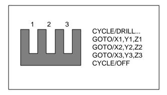
When a hole parameter changes, the CYCLE statement is restated with the changed parameters:
