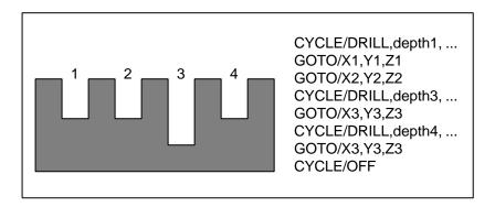
Each operation, prior to machining a series of holes, first positions to the clearance plane above the first hole. At the end of the series of holes, the CYCLE is canceled, and and a RAPID move is output to move the tool to the clearance plane above the final hole (it should be there anyway. This is done as a safety measure).
