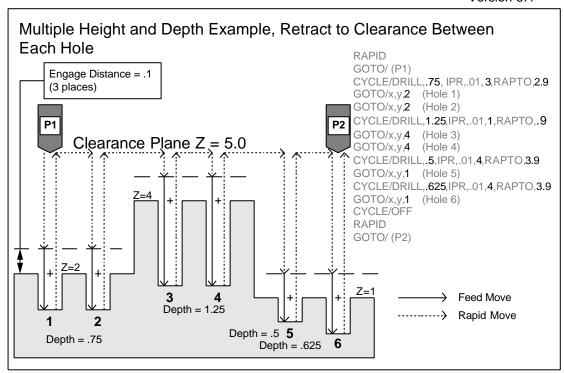
The option to have the tool retract only to clear obstacles is called "Retract to Minimum Z plus Clearance". When this option is used, the user specifies a clearance height, which is typically a small value. the tool will move at the user specified level above the holes unless there is an obstacle to be cleared or the next hole is at a different level.
