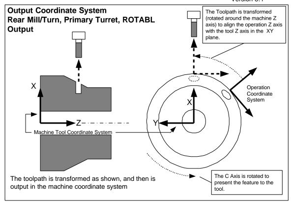
If the tool is tilted in the ZX plane, it is assumed that the tool holder is fixed at this angle or that the turning center has a programmable rotary head. The CLDATA is not altered or transformed based on the ZX plane angle.
