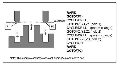
In Generative Machining holemaking operations, the user has a choice of using a single clearance plane that the tool retracts to after machining every hole, or having the tool retract only as far as necessary to clear an obstacle by the clearance value.
